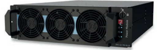
Power Module 67 kW (SiC) MP2 67 PM BLUE.
